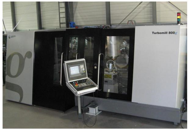
The LIECHTI Turbomill 800g is a highly dynamic five-axis milling machine with maximum axis acceleration, designed for high-speed milling in 5 axes.
